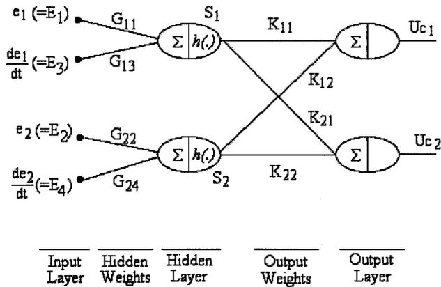
Fig. 9. NN2 structure for a 2-DOF robot to compute the corrective control [41].
