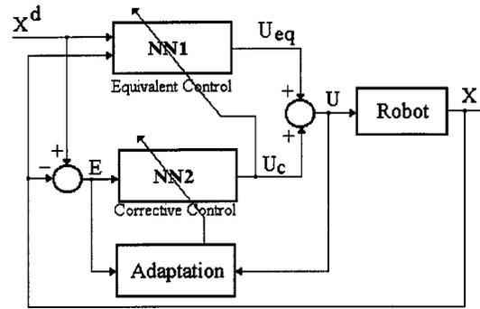
Fig. 7. The neuro-SMC architecture proposed by Ertugrul and Kaynak [41].
