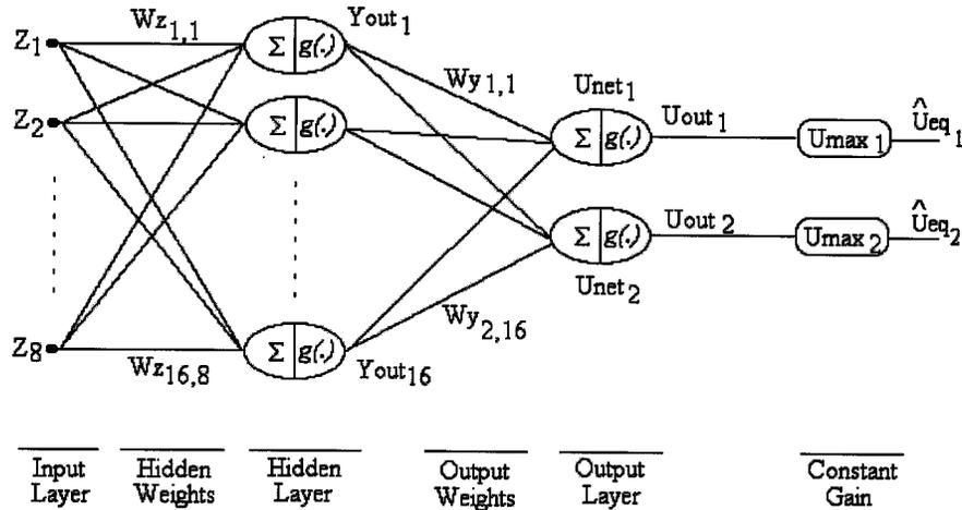
Fig. 8. NNI structure for a 2-DOF robot to compute the equivalent control [41].
