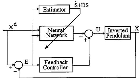
Fig. 10. Architecture proposed by Jezernik *et al.* [44].
