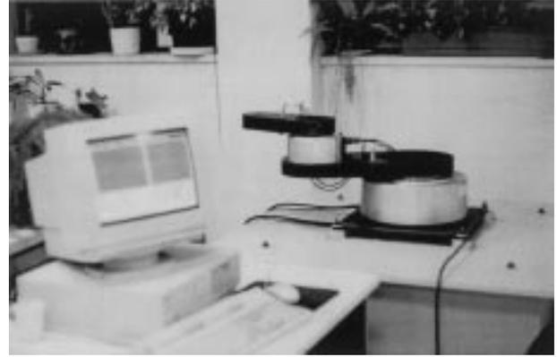
Fig. 2. Experimental two-link direct-drive arm.
