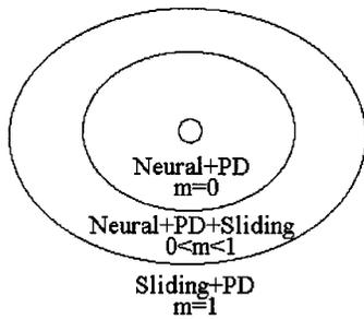
Fig. 12. Illustration of the activation scheme of the controllers based on the approximation error of the inverse dynamics [68].
