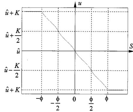
Fig. 4. Nonlinear operating line in an FSMC, resembling the saturation function used in conventional SMC.
