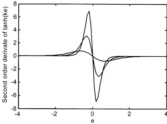
Fig. 4. The second order derivatives of  $\tanh(kx)$  (dashed line:  $k = 1$ , solid line:  $k = 2$ , dash-dot line:  $k = 3$ ).
