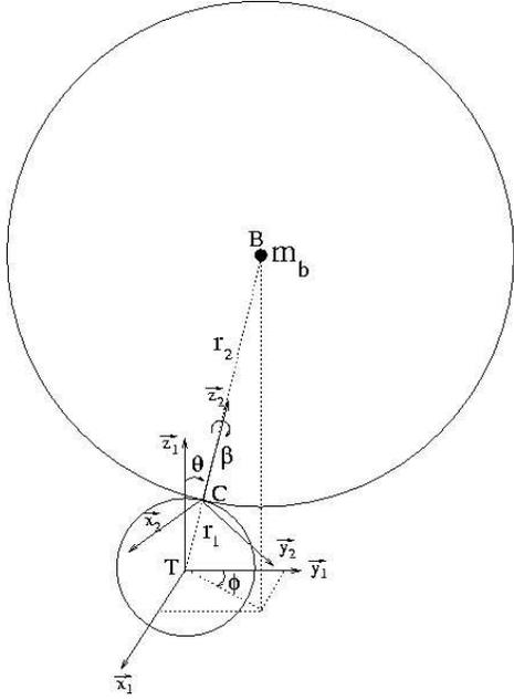
Fig. 2. Two balls with pure rolling constraint
