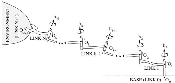
Fig. 1. N-link serial manipulator
