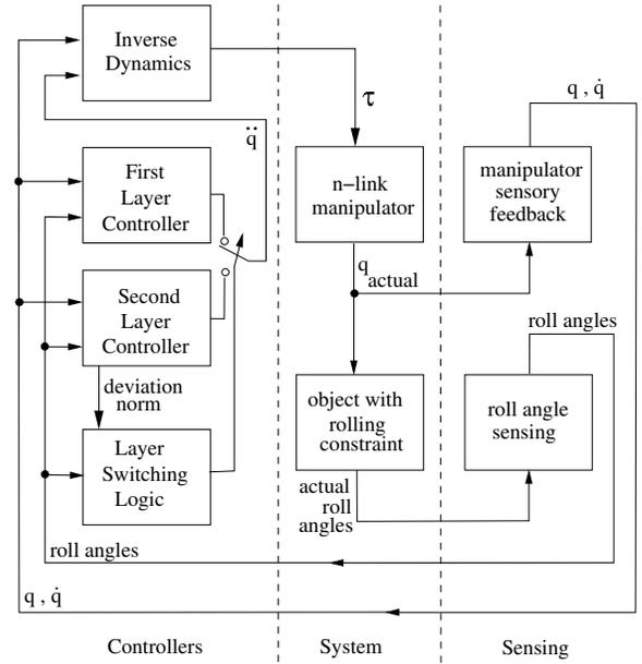
Fig. 6. High level schematic of the controller, system and sensing interaction
