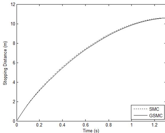
Fig. 4. Stopping distance of SMC and GSMC for a constant reference
