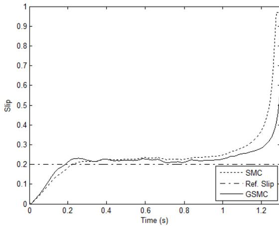
Fig. 3. Wheel slip of SMC and GSMC for a constant reference
