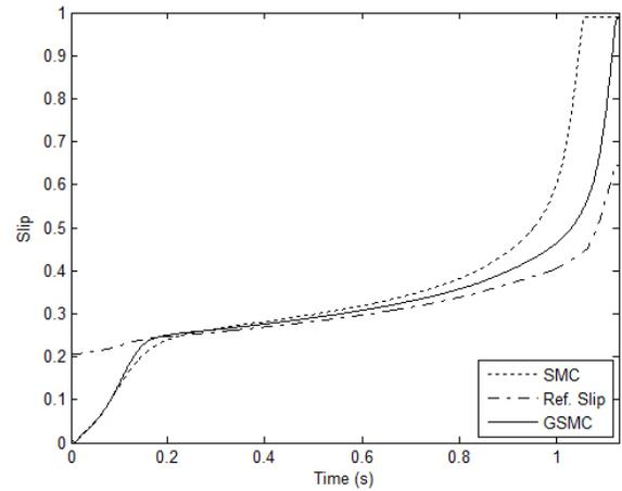
Fig. 5. Wheel slip of SMC and GSMC for a constant reference
