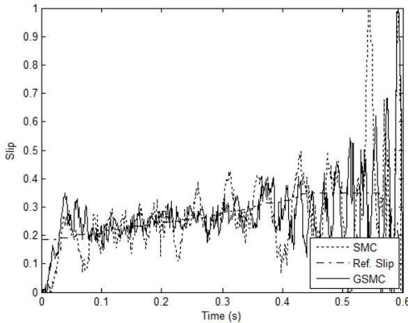
Fig. 8. Wheel slip of SMC and GSMC for velocity dependent reference
