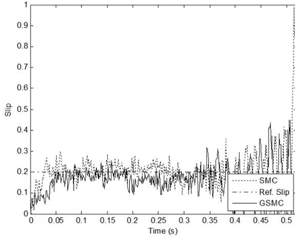
Fig. 7. Wheel slip of SMC and GSMC for constant reference
