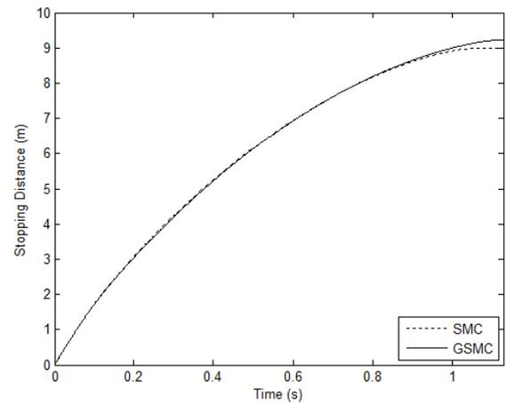
Fig. 6. Stopping distance of SMC and GSMC for velocity dependent reference
